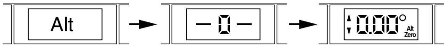
Press ALT ZERO again to return to standard reference mode. The Pro 3600 also returns to standard reference when it is turned off or shuts off automatically.
