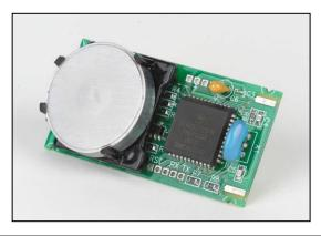
variety of applications, accept a standard 5 Volt DC supply, and provide both RS-232 and Pulse Width Modulated (PWM) outputs.
